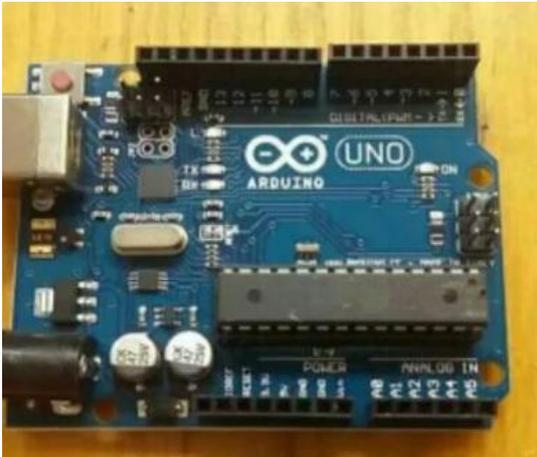
Gambar 2. 6 Pin Input/Output Arduino Uno
