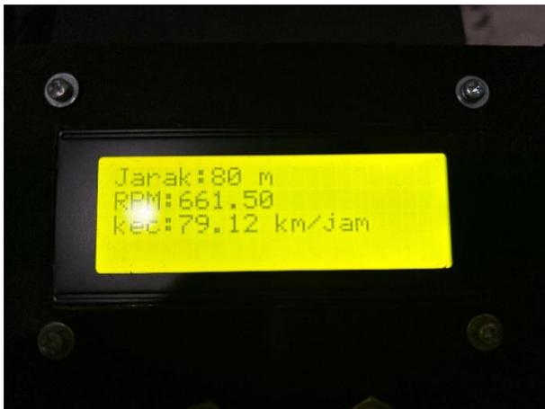
Gambar 2. 19 LCD 4x20
