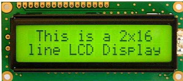
Gambar 2. 18 LCD 2x16
