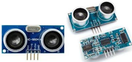
Gambar 2. 11 *Sensor Ultrasonic*
