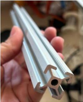
*Gambar 2. 14 Aluminium Profile T Slot*
