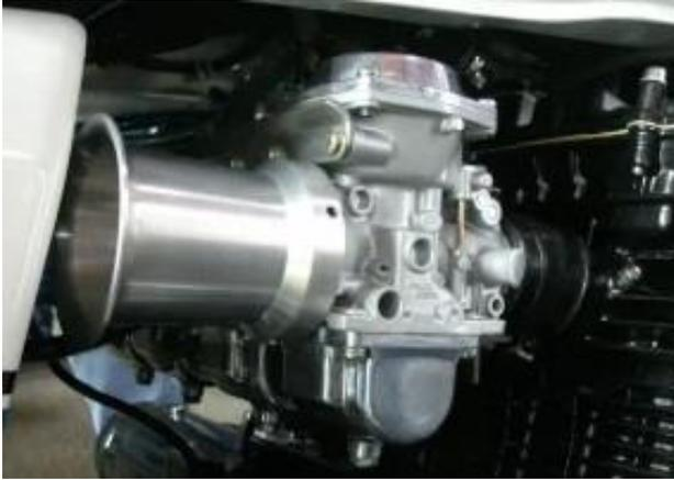
Gambar 2. 1 *Velocity Stack*
