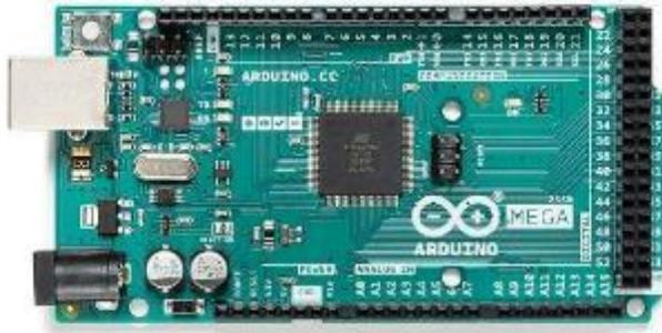
Gambar 2.3 Arduino Mega 2560
