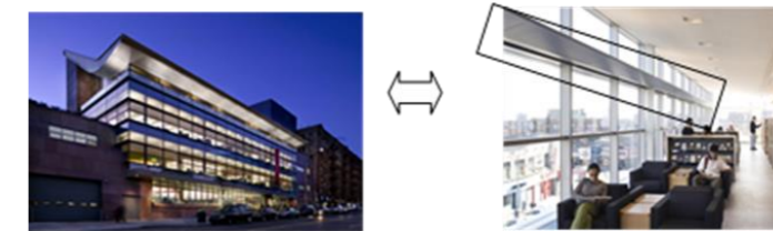
Gambar 2.17 Reflector light shelf pada ruang perpustakaan Sumber : https://www.dattner.com/projects/view/bronx-library-center/
